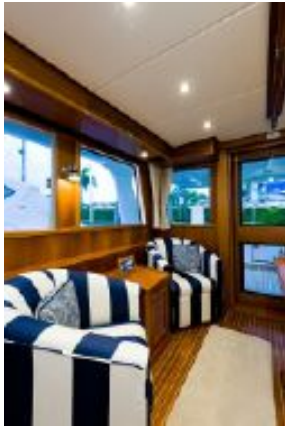
BONDED, DIRECT-GLAZE, FRAMELESS WINDOWS THROUGHOUT
